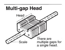
Then electrical techniques are used to separate the signals detected by the head and to output them as high-resolution digital signals.
