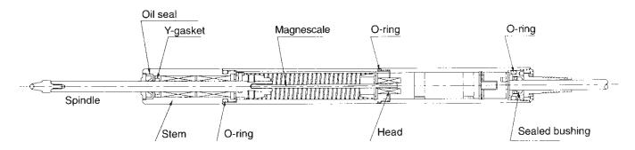
The Magnescale is a 2mm diameter rod made of ferromagnetic alloy recorded with 0.2mm pitch **magnetic graduations** (magnetization patterns). During manufacturing, the use of a special recording head and a **laser measuring** machine makes these graduations extremely accurate.
