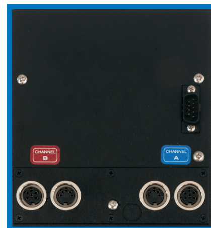
Rear of PRO-MIC Electronics with Temperature Inputs
