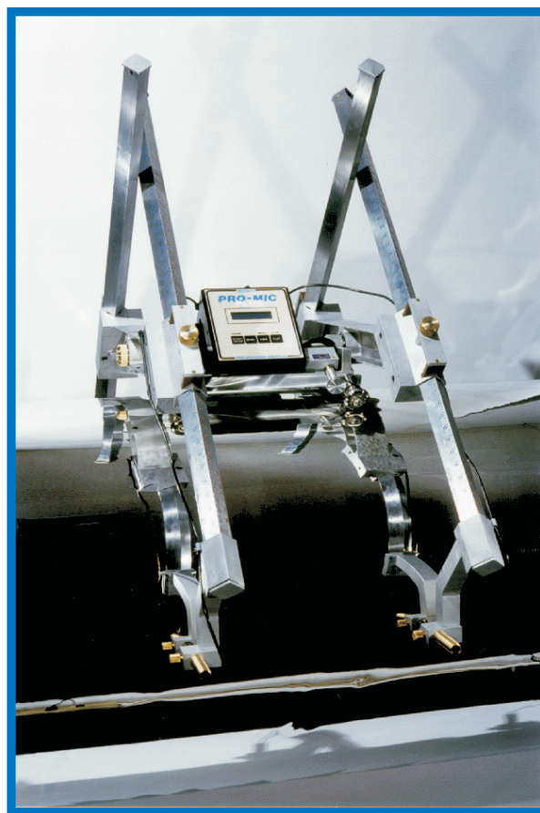
16" to 48" PRO-MIC TRUE End-to-End X-Caliper Design
