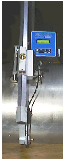
Opposed Probes for Rough Roll Surfaces
