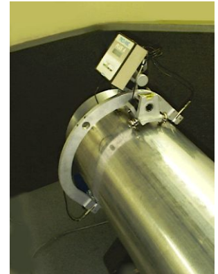
Stealth System at 45 Degrees for In Place Measurement
