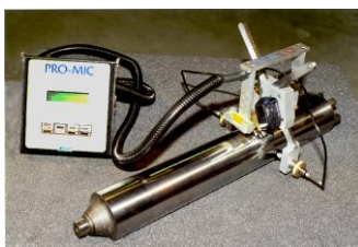
Z-Mill Opposed Probes to measure with Steady Rests in place
