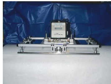
Alpine System to Detect Ridges in Rolls of Material
